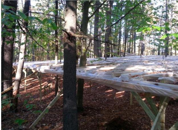
Fig.3. Example of a gutter lining the plot edge to collect and remove runoff at the Thompson Farm Drought Experiment, Durham, NH (photo credit: K. Jennings).
